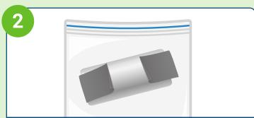
To prevent fires, tape battery terminals and/or place lithium-ion batteries in a separate bag. Keep batteries segregated from other materials.
