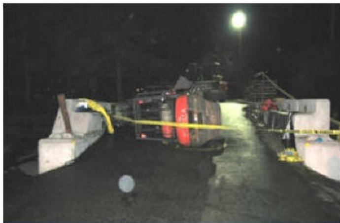
This photo shows the scene of a fatality that occurred when a forklift tipped over and the operator thought he could “jump clear.” He didn’t quite make it. He was crushed between the forklift rollover bar and the concrete floor. He wasn’t wearing his seatbelt.
